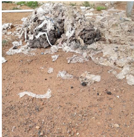
Monster blockage - caused by wet wipes - at Port Wakefield wastewater systems.
